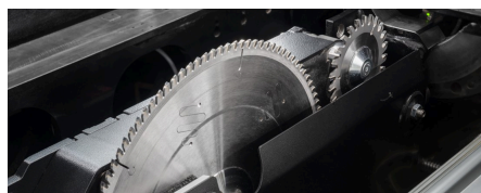
Scoring saw and main saw blade in a single pass
