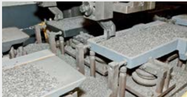
Surface scraping of cast iron table
