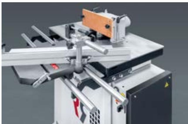
Cast iron tenoning table on heavy steel bars and tenoning hood for tools with diameter up to 250mm. (requires optional motor break)
