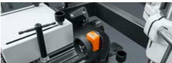
Micro adjustment and positioning by handwheel with mechanical counters. The topcover runs on ergonomic linear guides for easy reference and increased precision.
